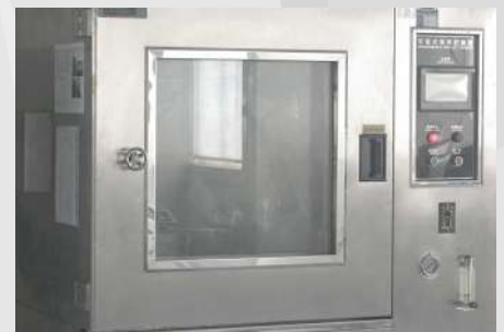
IPX5-6 Strong Water Spray Test
