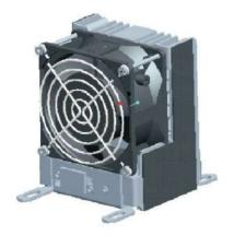
The product is composed of high-quality nickel-chromium alloy heat pipe, die-casting aluminum structure heat sink, high-performance axial fan, and temperature control switch. The electric heat pipe is placed in the center of the radiator body. The temperature control switch is near the electric heat pipe and hidden in the radiator body. The axial flow fan is close to the loose body.
