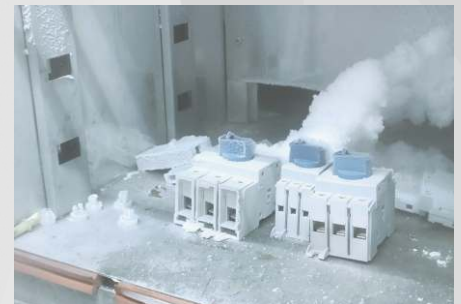
High Low-Temperature Humid-Heat Test
